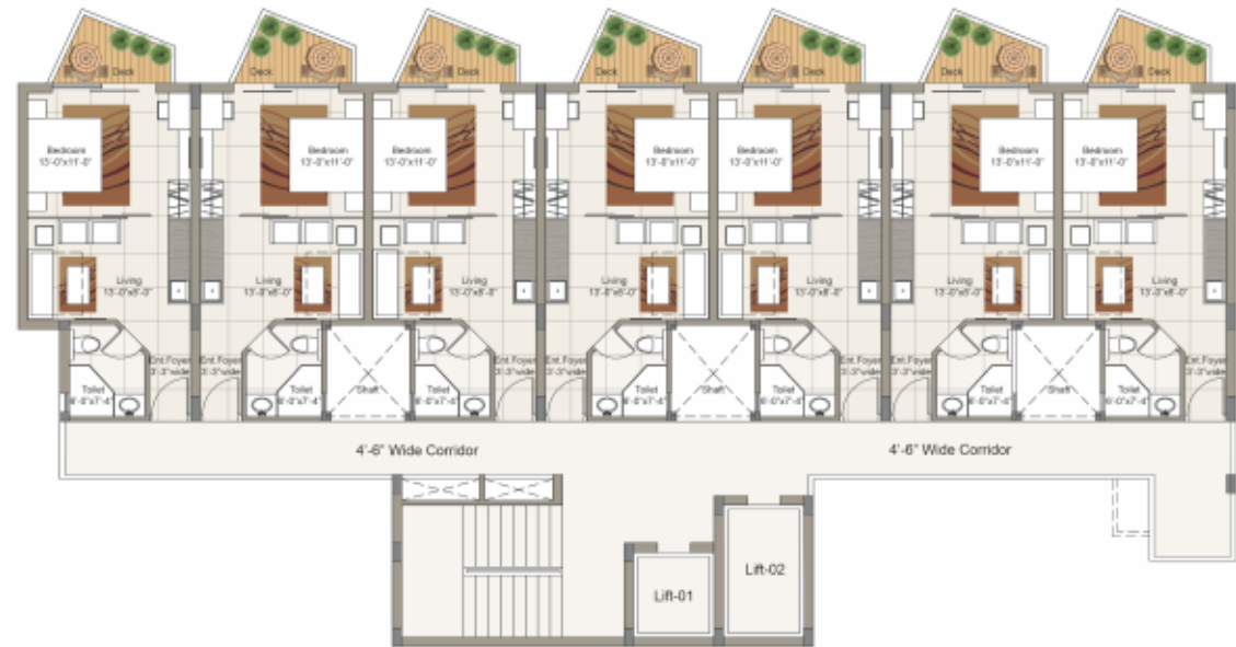
TYPICAL 1ST TO 6TH FLOOR PLAN FOR BLOCK C (STUDIO / 1BR CLUSTER)
