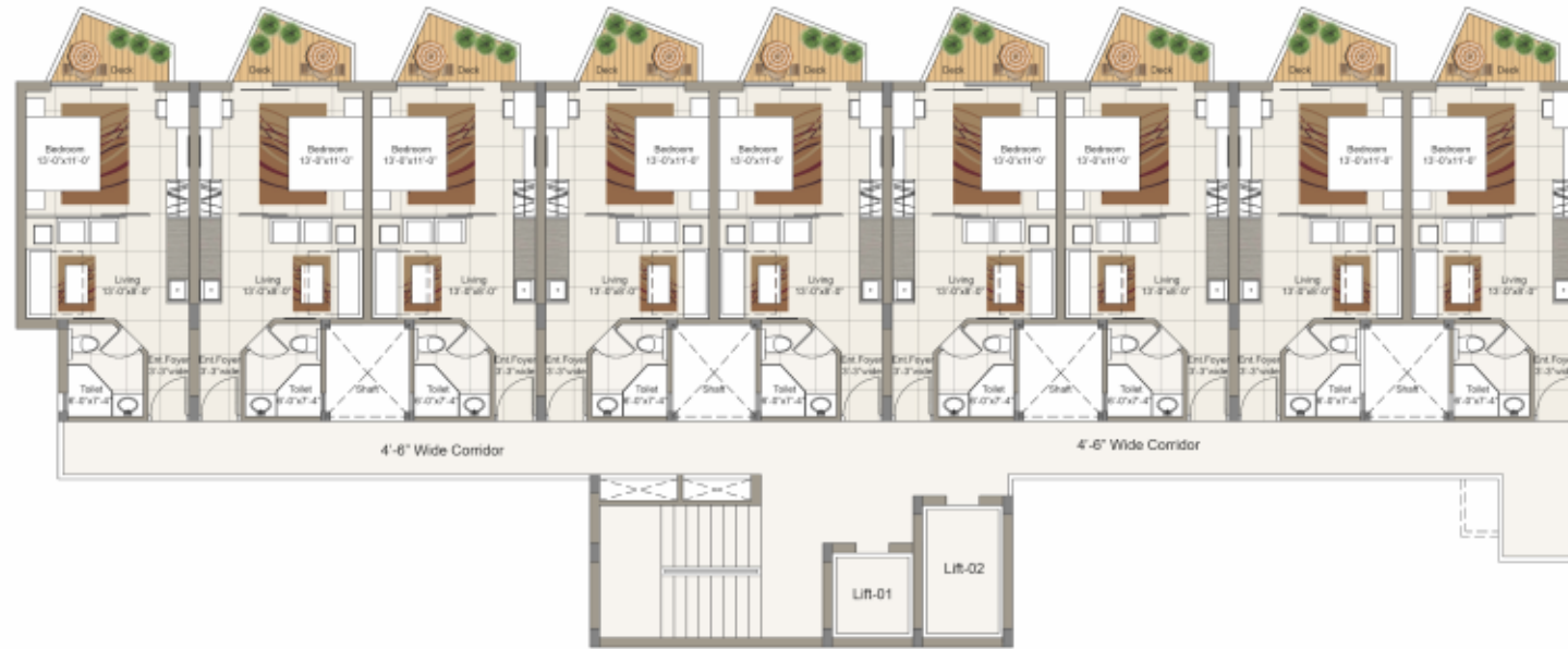
TYPICAL 1ST TO 6TH FLOOR PLAN FOR BLOCK B (STUDIO / 1BR CLUSTER)
